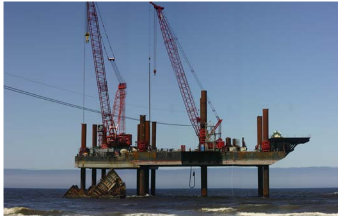
Barge with cranes held aloft on jacks.
