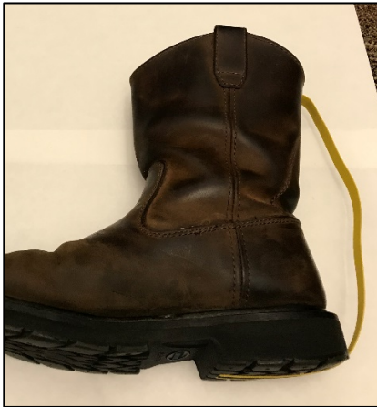
Figure VIII-3: Heel grounders. (Source: OSHA HRT)
