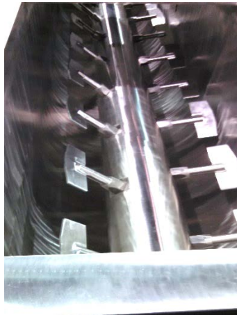
Single Rotor Paddle Mixer (Source: R5)
