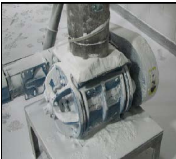
Figures 2: Dust accumulation on a fan blower. (Source: OSHA HRT)
