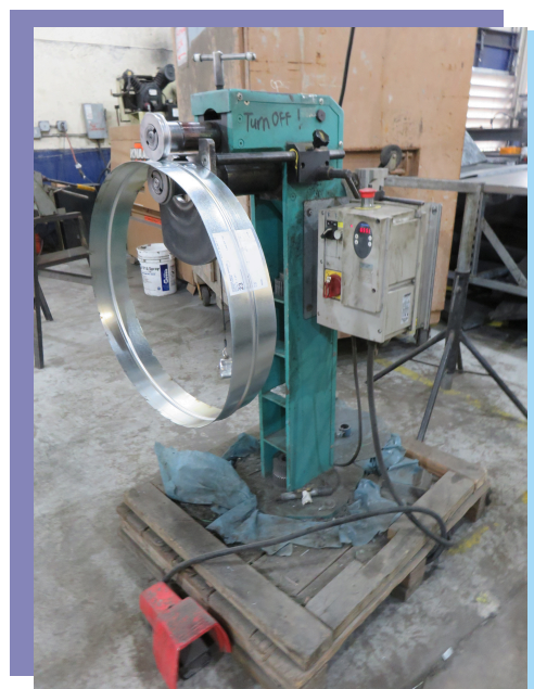
Image of a swaging machine with the circular metal coupling ring between the two dies.
